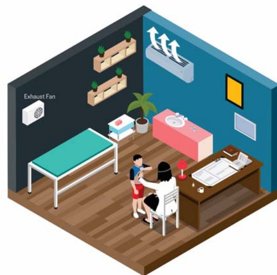
Fig. 2 Clinic setting - Placement of exhaust fan, one feet above the ground. Direction of air should be from clean to dirty (patient side). Flow of AC air should be directed towards ceiling.
